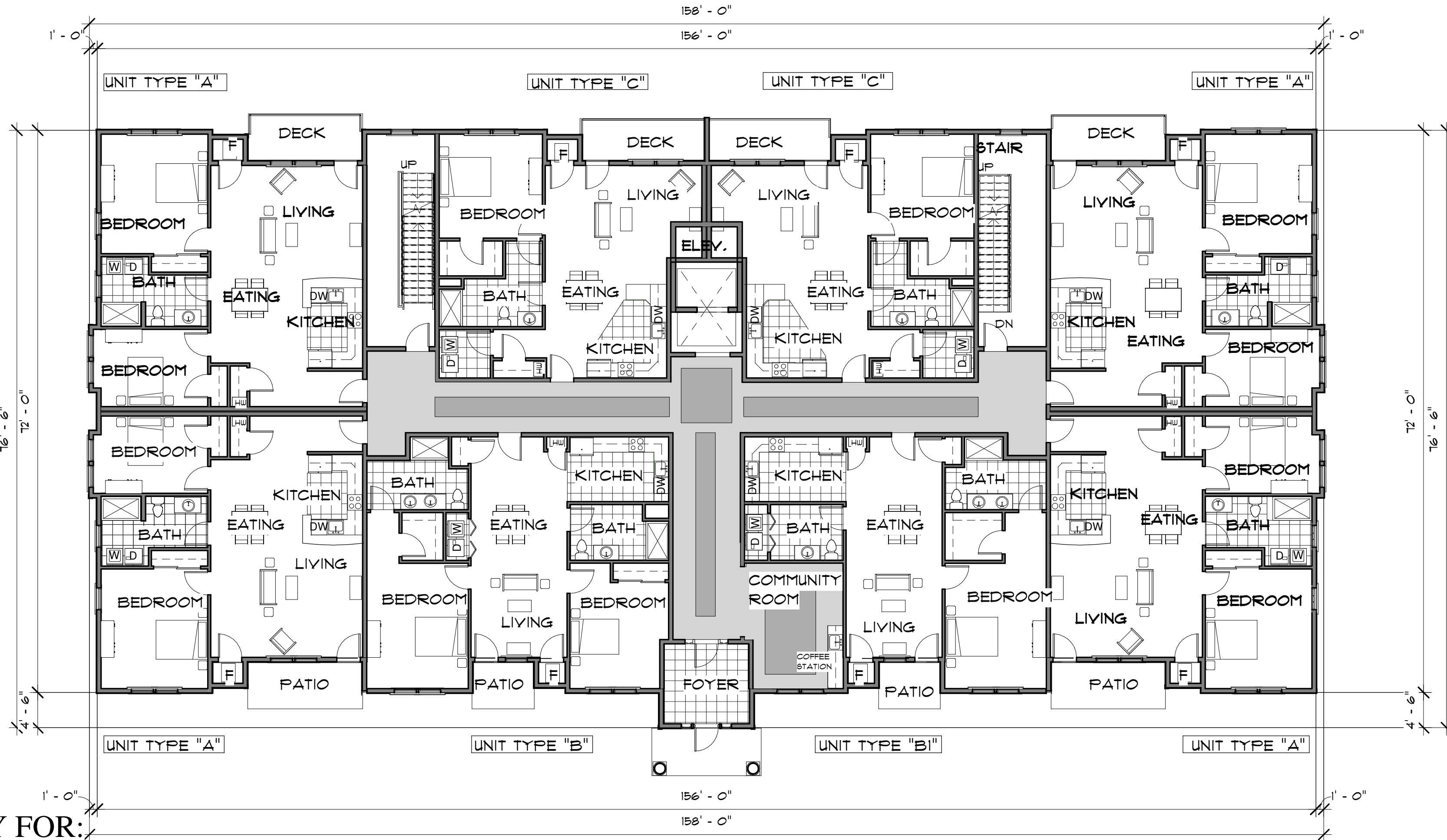
1 FIRST FLOOR PLAN. 3/32" = 1'-0"
