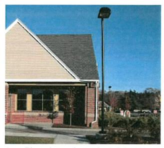
A cut-off fixture that complements the simple line of this commercial building. The fixture is mounted on an 18-foot pole on a one-foot base for an effective height of 19 feet.
