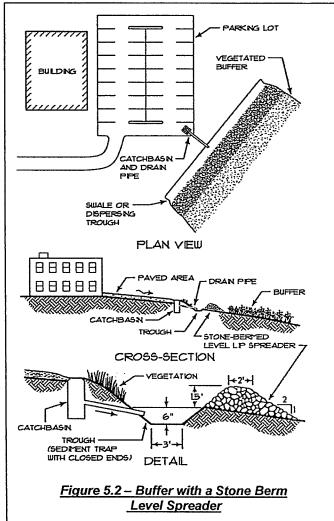
be applied in the design and construction of a buffer with a stone bermed level lip spreader.
