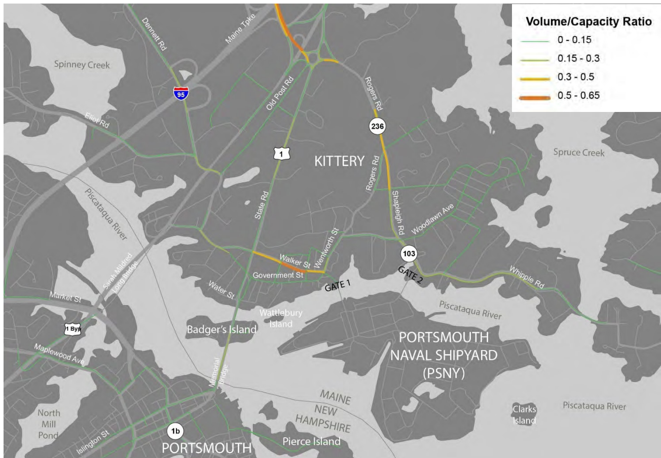
Figure 8. Walker Street nearest Gate 1 has a higher ratio of Volume to Capacity but still doesn't exceed capacity. The majority of roads in Kittery are operating well under capacity.
