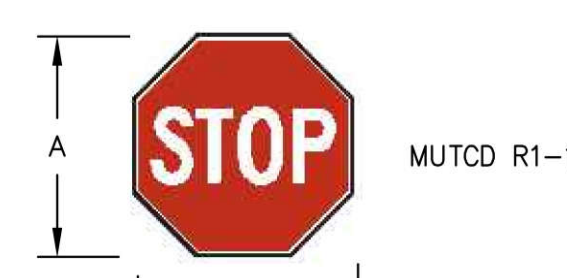
STOP SIGN (R1-1) NOT TO SCALE NOTES: 1. WHITE LEGEND & BORDER ON RED BACKGROUND 2. SIGN SHALL BE RETROREFLECTIVE 3. SIGN SHALL COMPLY W/ MUTCD STANDARDS DIMENSIONS 4. A = 30" FOR SIGN AT CAR WASH DRIVEWAY 5. A = 36" FOR SIGN ON MACKENZIE LANE
