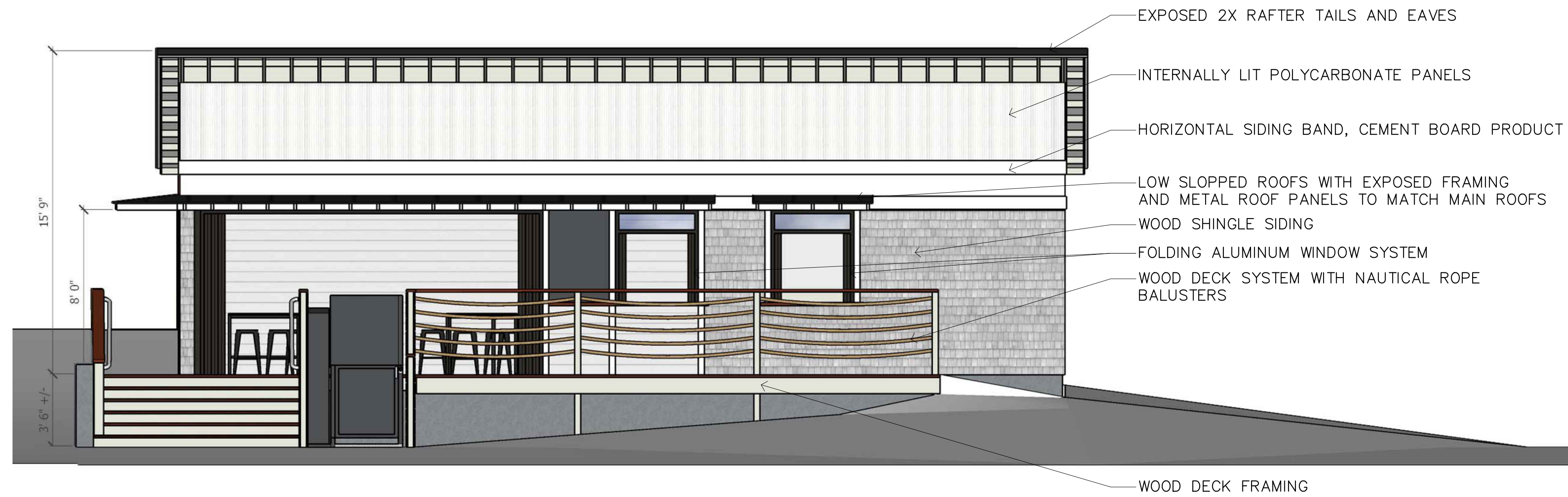
FRONT ELEVATION SHOWING DECK SCALE: 1/4"=1'-0" PB.2 1
