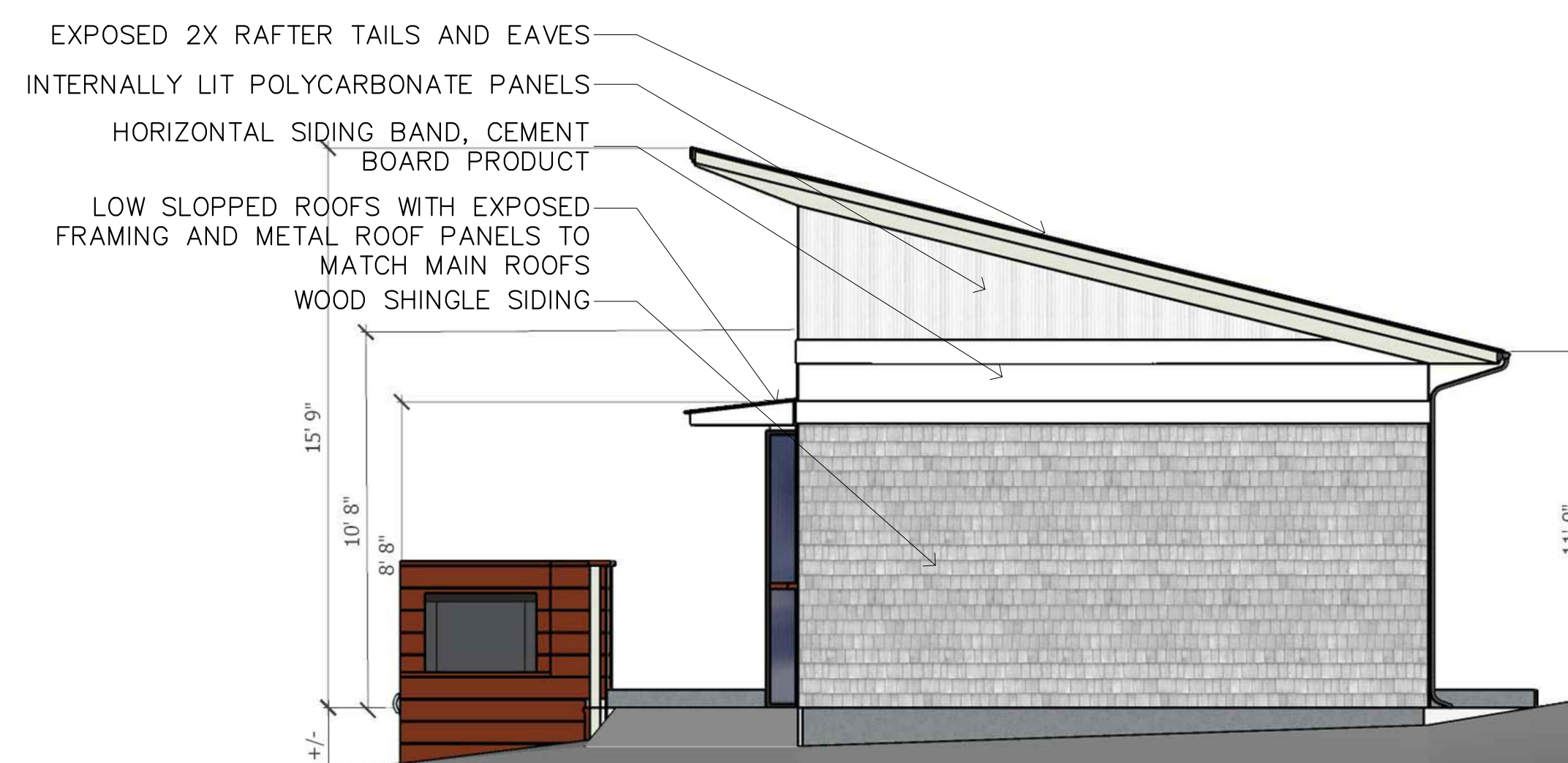
WEST ELEVATION SCALE: 1/4"=1'-0" PB.2
