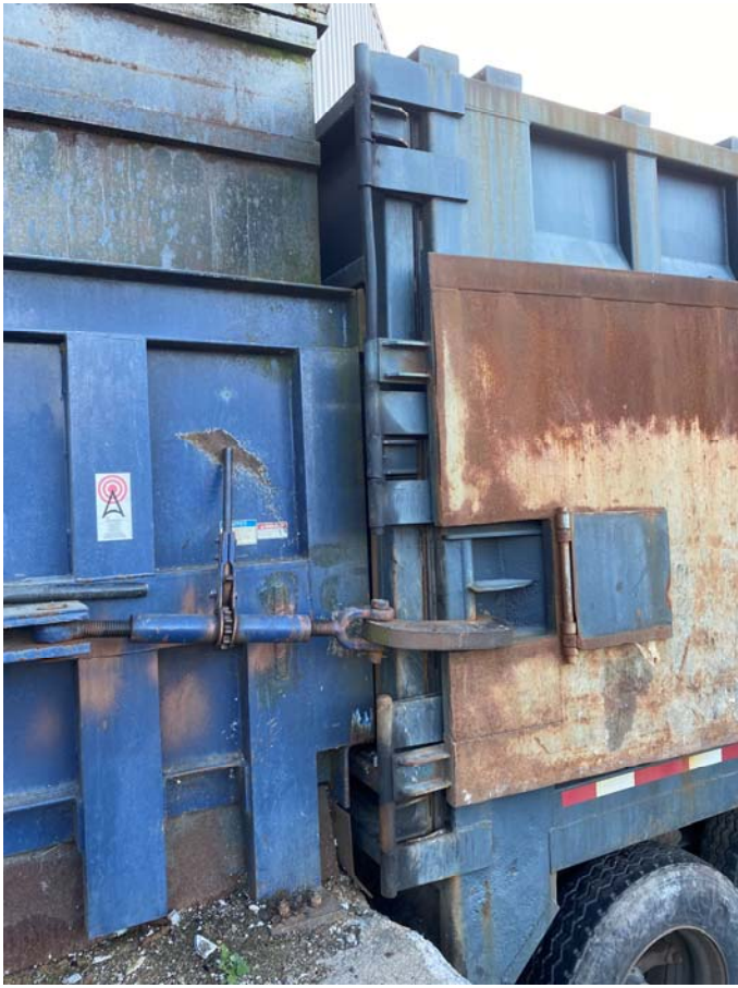
Existing Municipal Solid Waste Trailer & Chute Connection
