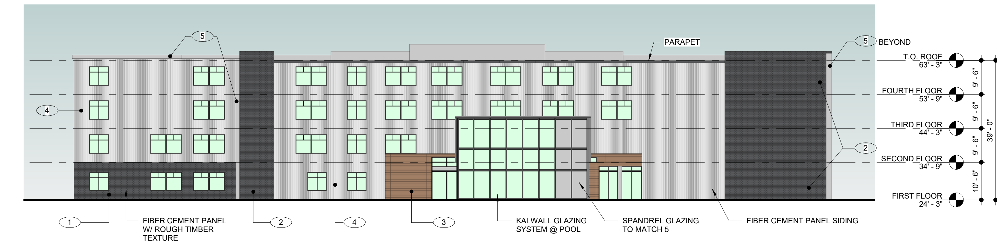
3 PROPOSED EXTERIOR ELEVATION - NORTH SCALE: 1/16" = 1'-0"
