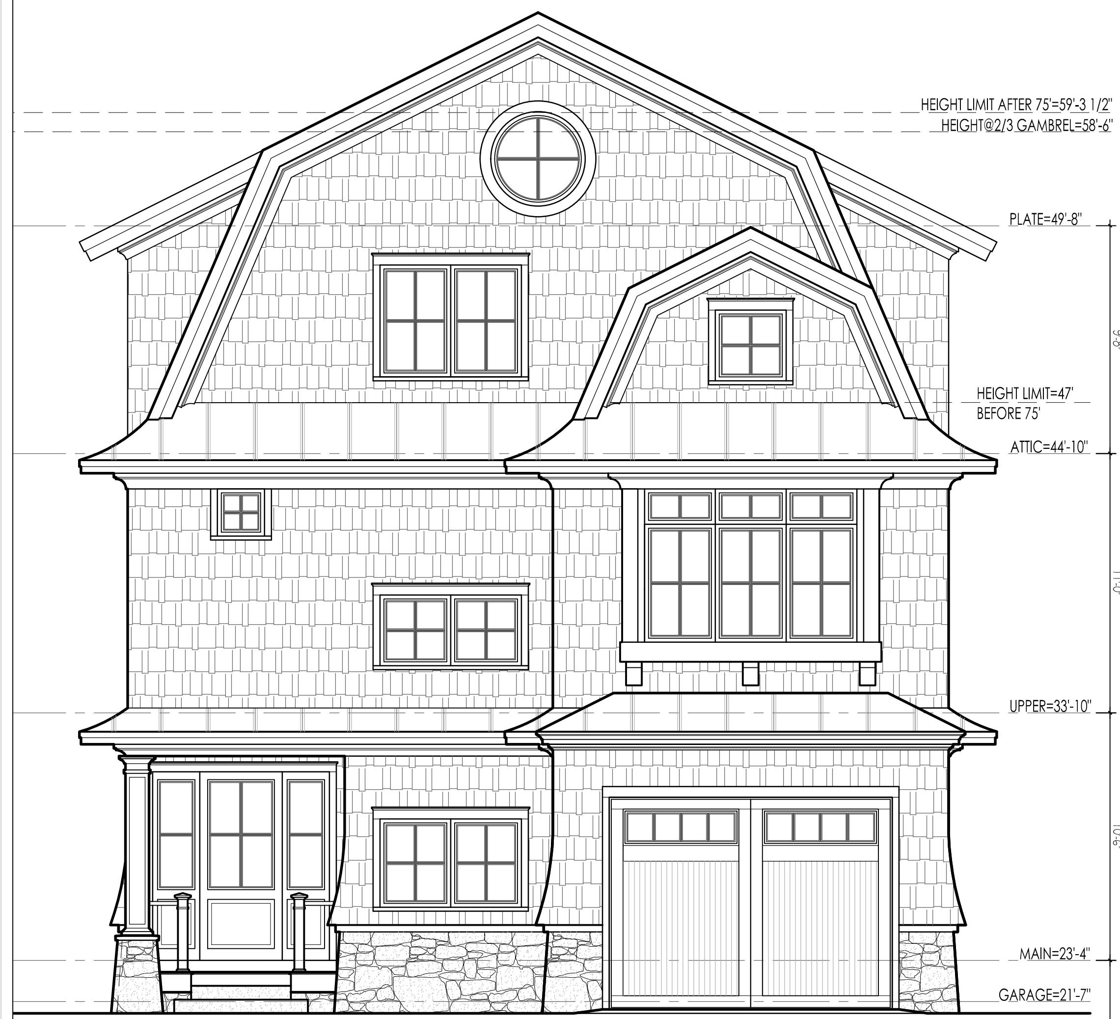
2 NORTH EXTERIOR ELEVATION SCALE 1/4" = 1'-0"
