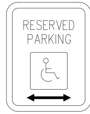
R7-8 SIGN R7-8 AS SHOWN IN THE MUTCD. INSTALLATION WILL BE IN ACCORDANCE WITH THE MUTCD AND MDOT STANDARD SPECIFICATIONS SECTION 719 - SIGNING MATERIAL.
