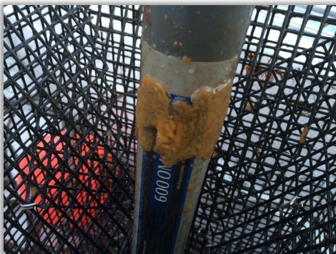
The middle estuary sonde was deployed in an eel trap (top); tunicates were found only on the sonde casing (left) with some algae coatings on the sensors (right).
