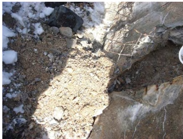
Figure 25: Weathering of Paste as seen through Chiseling
