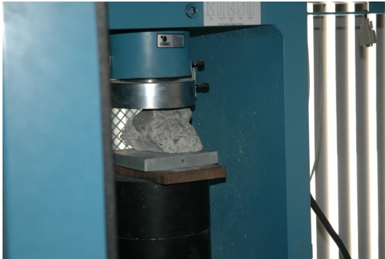
Figure 46: Hydraulic Crushing Machine
