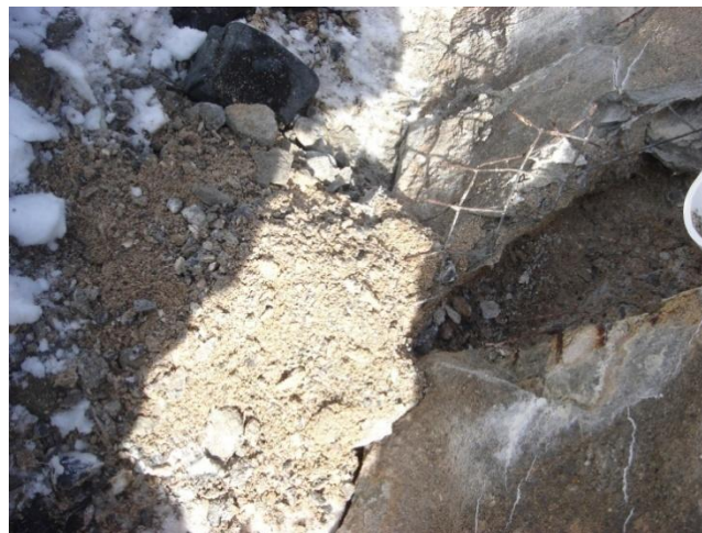
Figure 25: Weathering of Paste as seen through Chiseling
