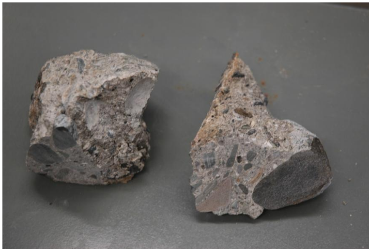
Figure 47: Core Sample after Fracture
