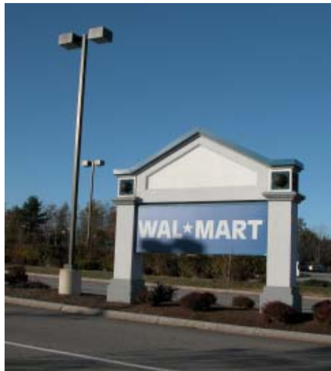
Simple 'shoe-box' fixtures mounted on square poles provide a clean look that complements the site.
