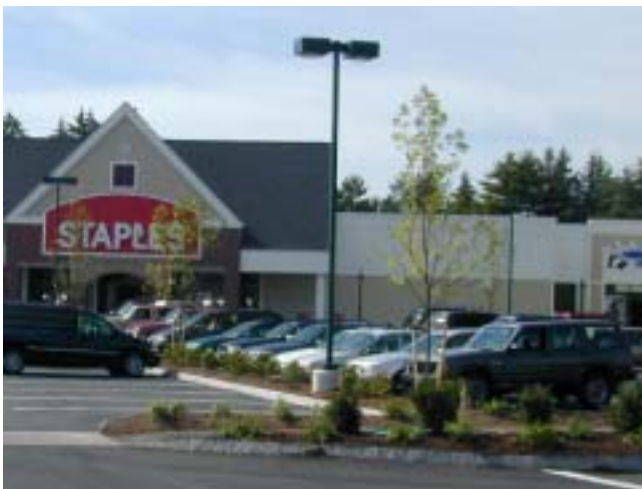
These light fixtures have been coordinated with the planting plan to avoid problems as the trees mature. Slightly raised bases protect the poles from plow damage.
