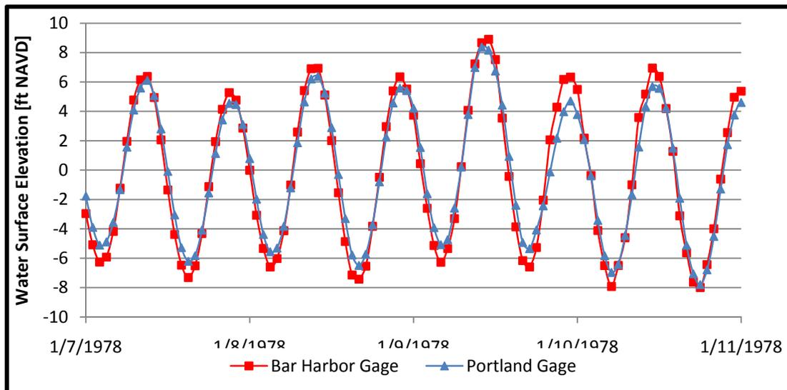
Figure 2-11 : Water Surface Elevation Data from the Bar Harbor and Portland Tide Gages for the January 9, 1978 Storm Event
