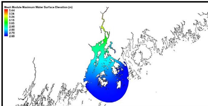
Figure 3-10 : Maximum Stillwater Level in the Penobscot RMA2 Model
