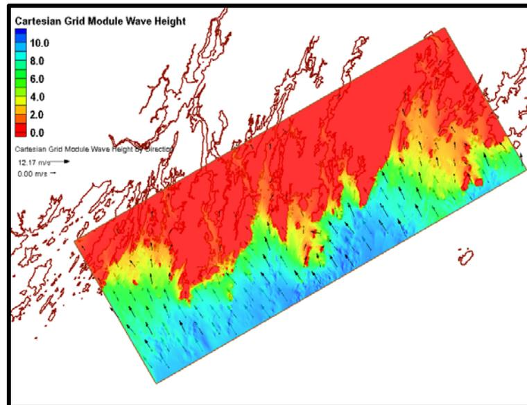
**Figure 4-19 : Lincoln-Sagadahoc STWAVE Grid Wave Heights (meters) and Direction Resulting from the 1-Percent-Annual-Chance Storm Simulation**
