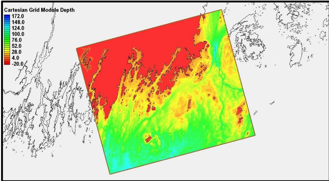
Figure 4-7 : Extent and Depth Contours for the Knox STWAVE Grid (meters)<sup>1</sup>
