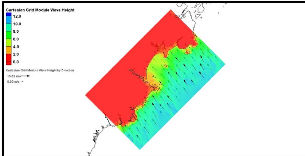
**Figure 4-21 : Biddeford STWAVE Grid Wave Heights (meters) and Direction Resulting from the 1-Percent-Annual-Chance Storm Simulation**
