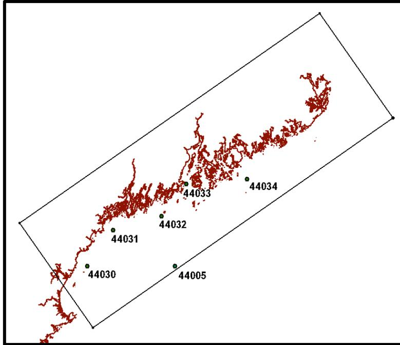
Figure 4-13 : Locations of Buoy 44005 Used for Establishing Boundary Conditions and Buoys 44030, 44031, 44032, 44033 and 44034 Used for Validation of the December 2007 Storm Event
