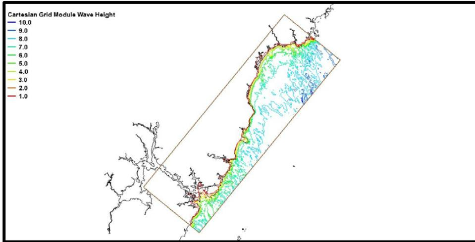
**Figure 4-22 : Wells STWAVE Grid Wave Heights (meters) and Direction Resulting from the 1-Percent-Annual-Chance Storm Simulation**
