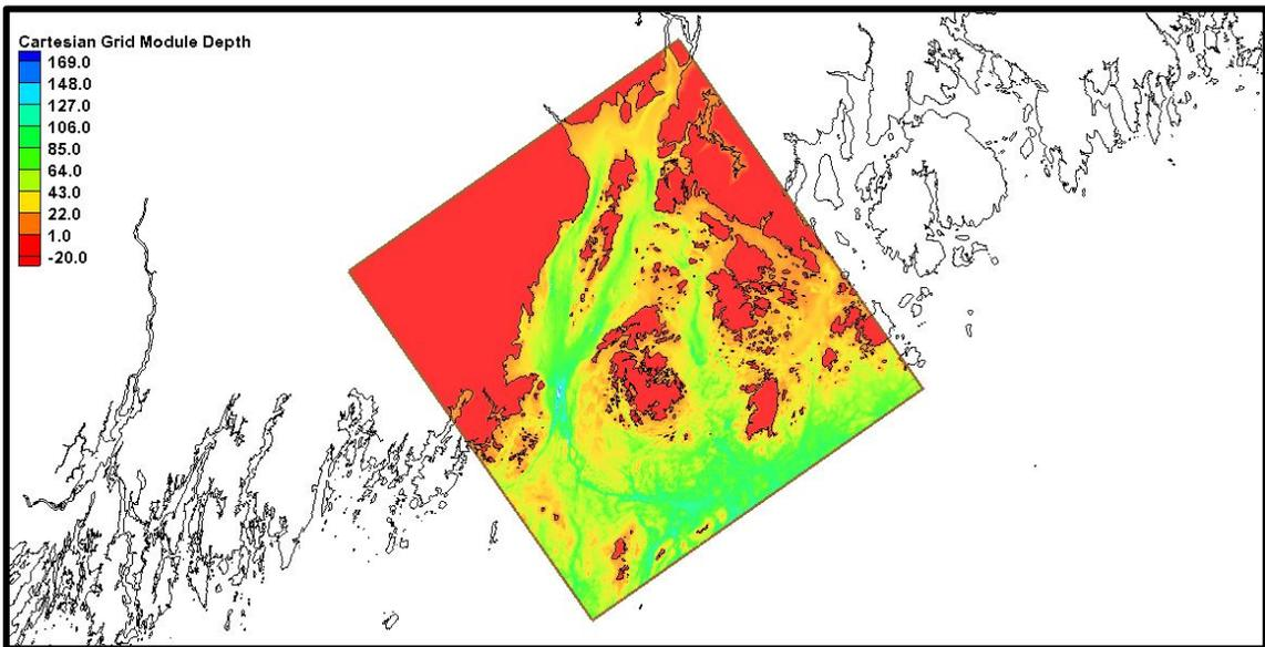
Figure 4-6 : Extent and Depth Contours for the Penobscot Bay STWAVE Grid (meters)
