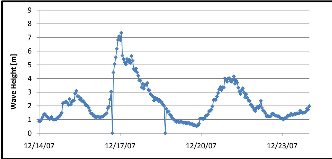
**Figure 2-12 : Wave Height Recorded at NDBC Buoy 44005 During December 2007 Storm Event**
