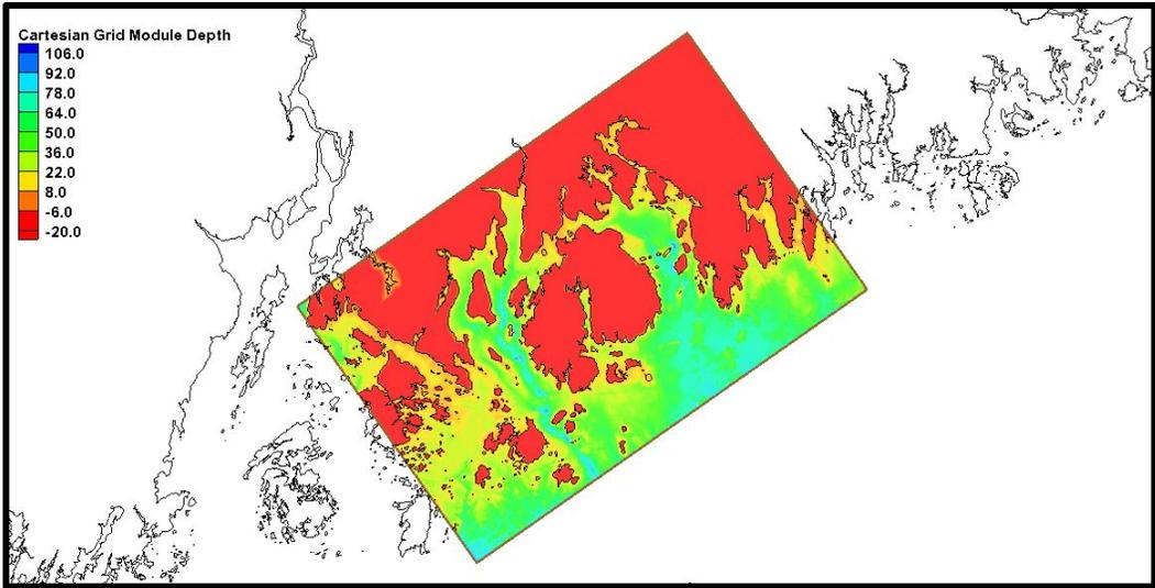
Figure 4-5 : Extent and Depth Contours for the Hancock STWAVE Grid (meters)
