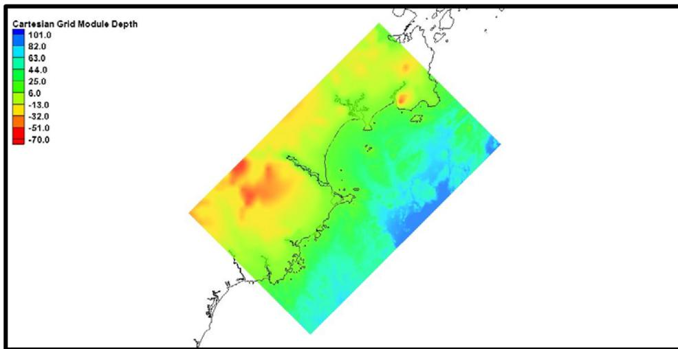
Figure 4-10 : Extent and Depth Contours for the Biddeford STWAVE Grid (meters)
