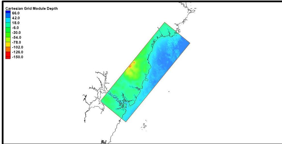
Figure 4-11 : Extent and Depth Contours for the Wells STWAVE Grid (meters)
