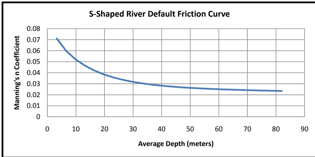
**Figure 3-5 : Automatic Roughness by Depth Default Curve as defined in RMA2**
