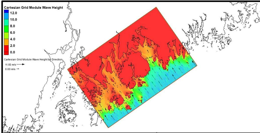
**Figure 4-16 : Hancock STWAVE Grid Wave Heights (meters) and Direction Resulting From the 1-Percent-Annual-Chance Storm Simulation**
