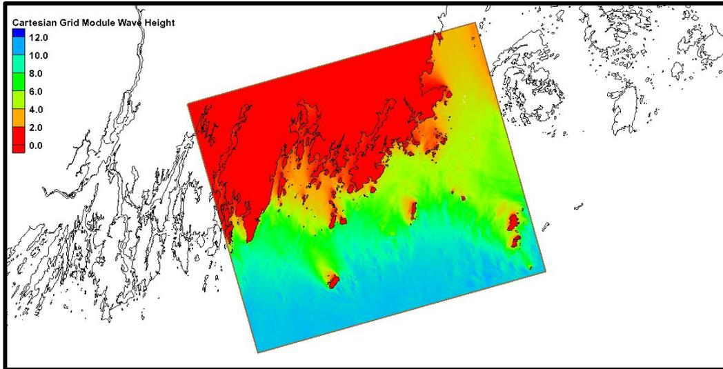
**Figure 4-18 : Knox STWAVE Grid Wave Heights (meters) and Direction Resulting from the 1-Percent-Annual-Chance Storm Simulation**
