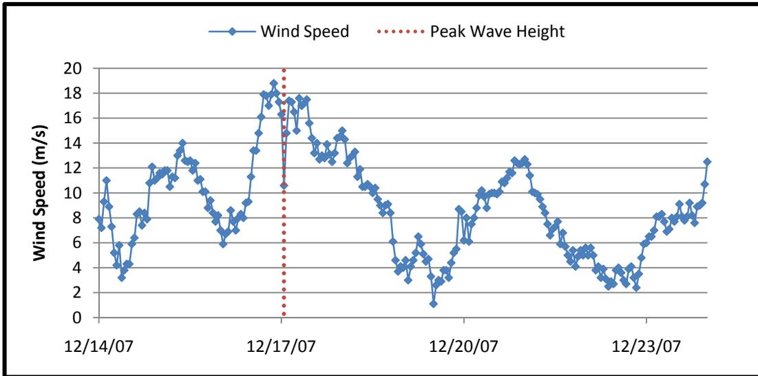
Figure 2-15 : Wind Speed Recorded at NDBC Buoy 44005 During December 2007 Storm Event
