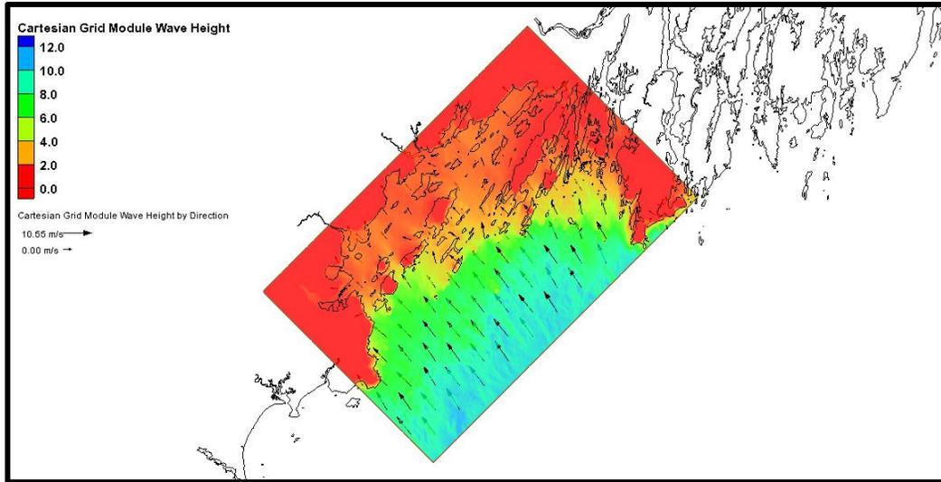
**Figure 4-20 : Casco Bay STWAVE Grid Wave Heights (meters) and Direction Resulting from the 1-Percent-Annual-Chance Storm Simulation**
