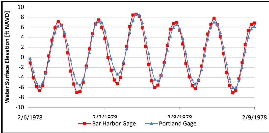
Figure 2-10 : Water Surface Elevation Data from the Bar Harbor and Portland Tide Gages for the February 7, 1978 Storm Event
