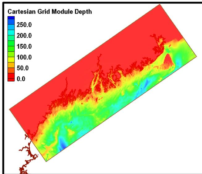
Figure 4-2 : Extent and Depth of the Coarse STWAVE Grid (meters)
