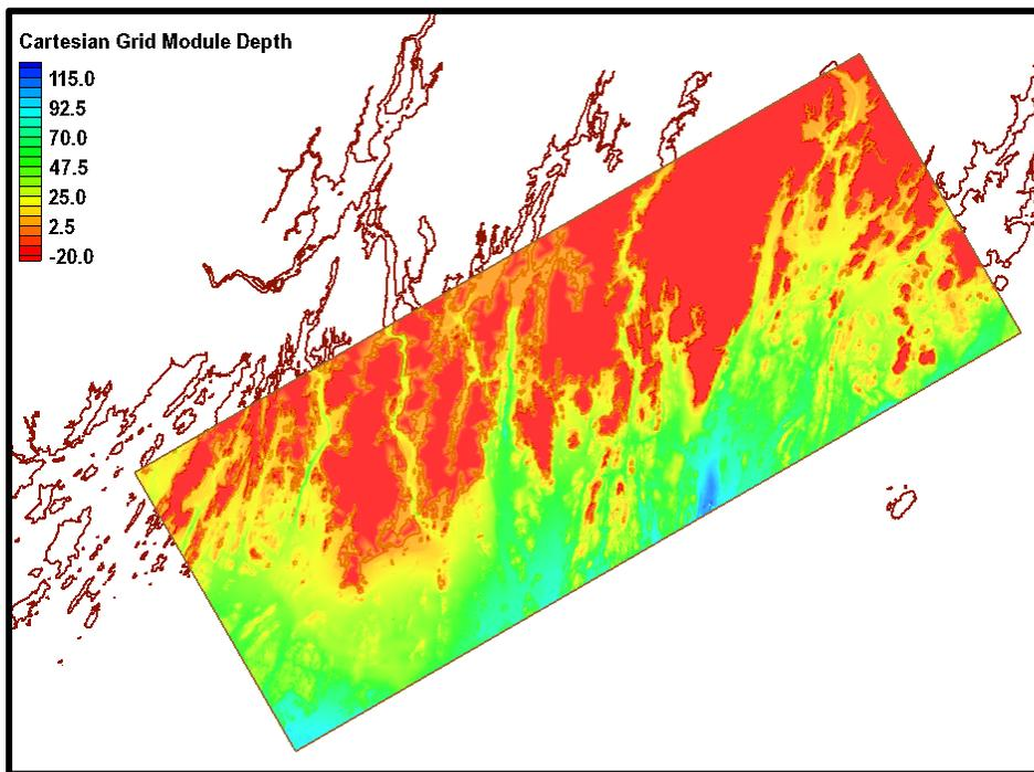
Figure 4-8 : Extent and Depth Contours for the Lincoln-Sagadahoc STWAVE Grid (meters)
