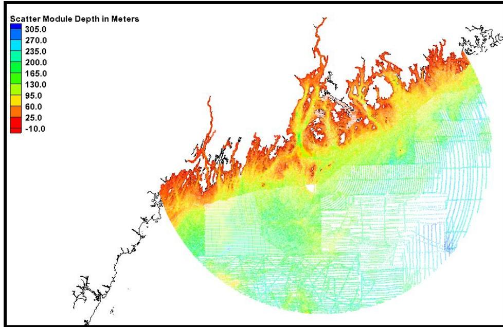
Figure 2-1 : Bathymetry Scatter Dataset Used for RMA2 Mesh
