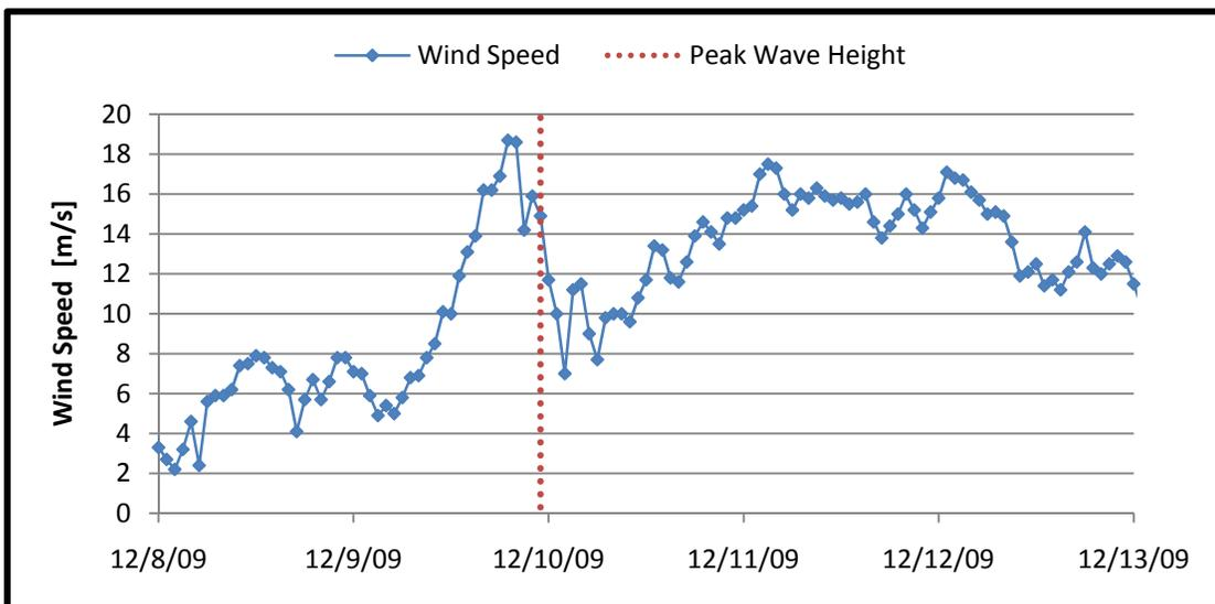
Figure 2-14 : Wind Speed Recorded at NDBC Buoy 44005 During December 2009 Storm Event
