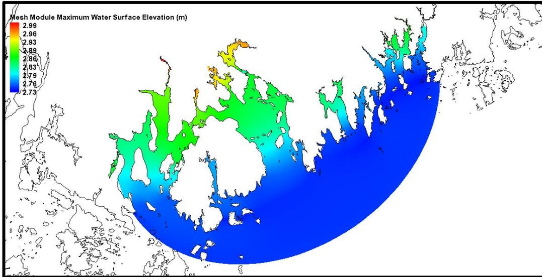
Figure 3-11 : Maximum Stillwater Level in the Eastern RMA2 Model
