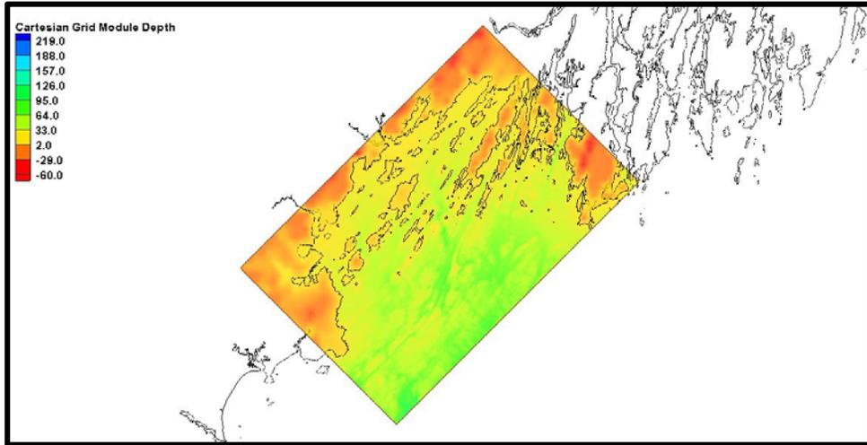
Figure 4-9 : Extent and Depth Contours for the Casco Bay STWAVE Grid (meters)
