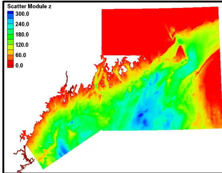
**Figure 2-2 : 200 Meter Resolution Bathymetry Raster Dataset Used for STWAVE Coarse Grid**
